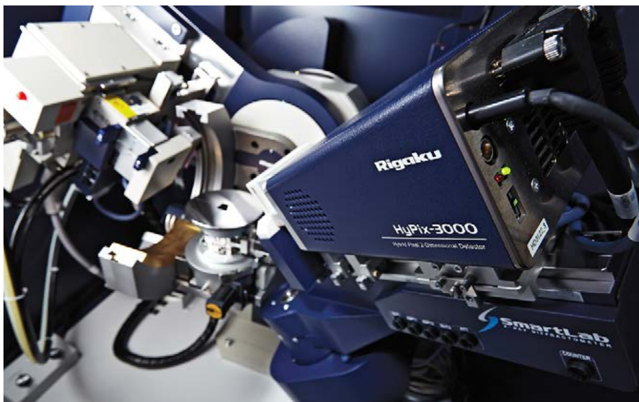
Kamera HyPix-3000 zamontowana na ramieniu dyfraktometru HyPix-3000 camera mounted on diffractometer arm
