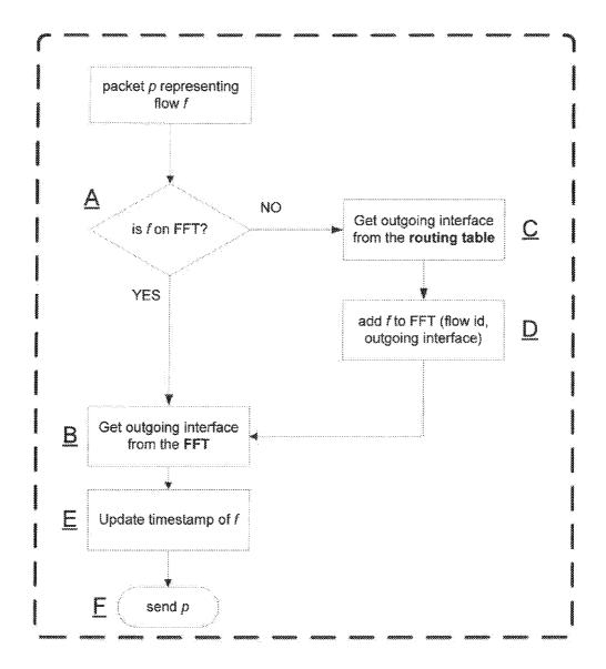
Fig. 3 Block diagram of the Output Interface Selector
